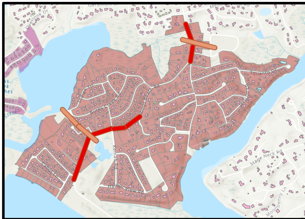
Figure 10. Approximately 423 properties (in dark brown) isolated by a flooded Hardings Beach Road (in red). Note proposed culverts in brown.
