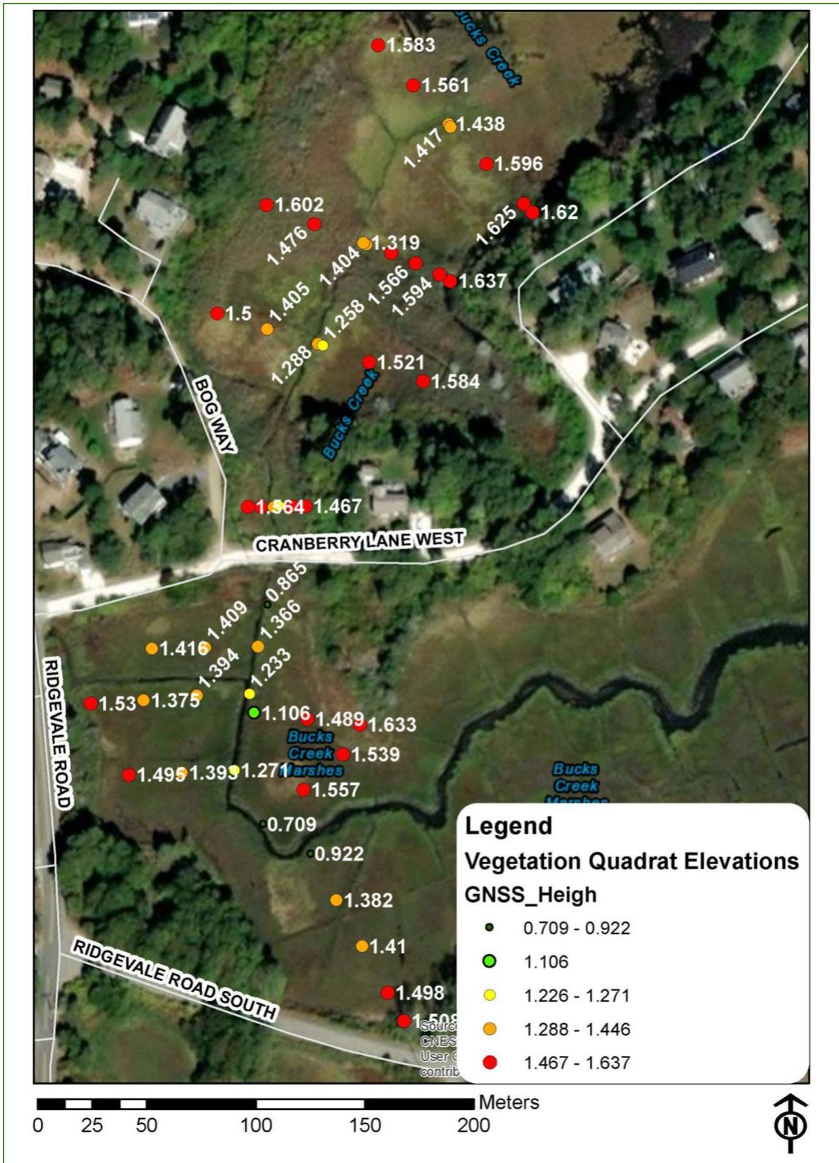
Figure 19: Map displaying the location and elevation (including 0.9m offset) of the quadrats on Bucks Creek north and south of Cranberry Lane.
