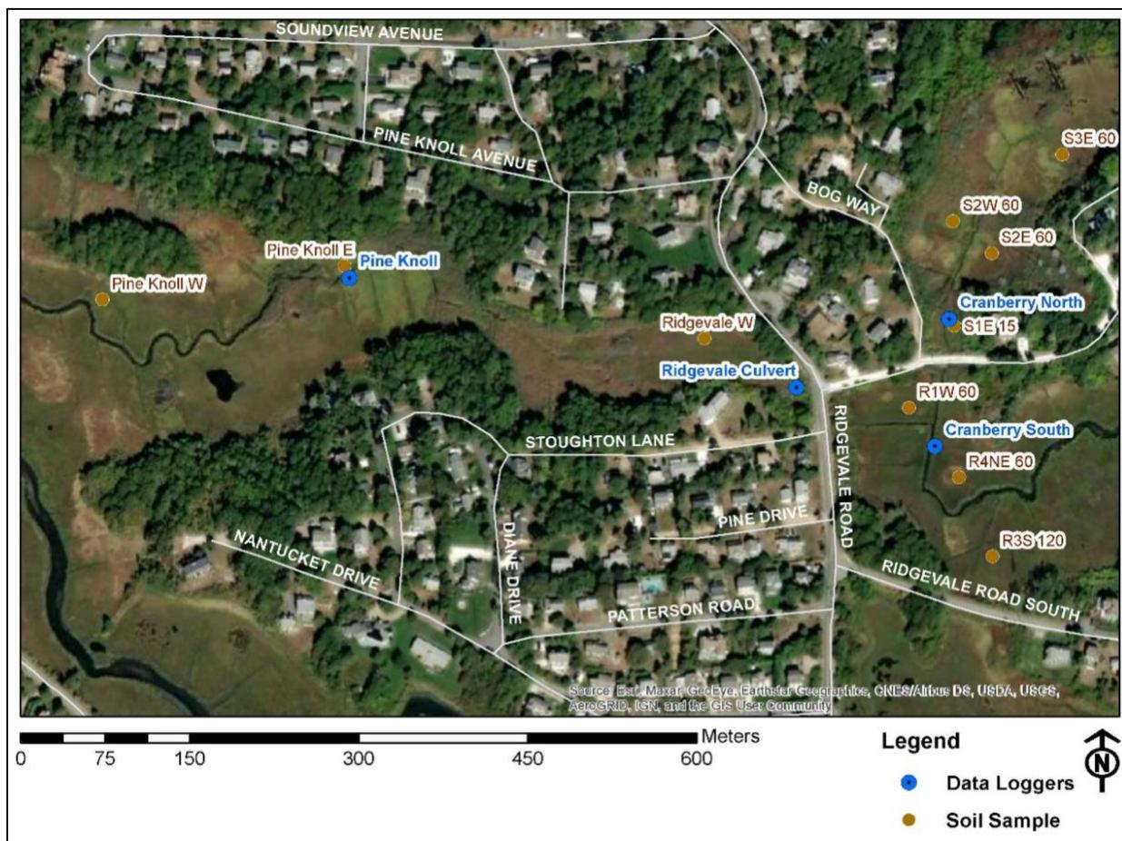
Figure 2: Map of the water level and salinity logger placement and soil sample sites (not shown: Barn Hill soil samples).
