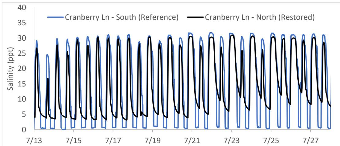
Figure 9: Salinity data collected from automated data loggers within the tidal creek north and south of Cranberry Lane. The time series shows the impact of a neap tide (7/13 – 7/20) and spring tide (7/21 – 7/28) on salinity concentrations in the restored (north) and reference (south) areas surrounding Cranberry Lane.
