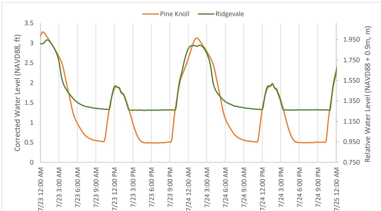
Figure 8: Pine Knoll East and Ridgevale West water level data spanning two full tidal cycles.
