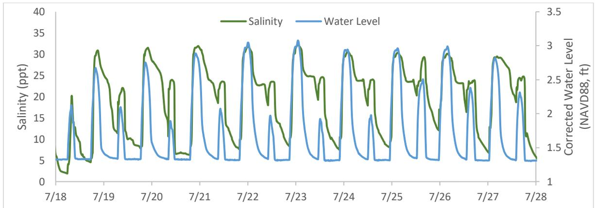
Figure 11: Salinity and water level during a spring tide at the marsh located on the western side of Ridgevale Road.
