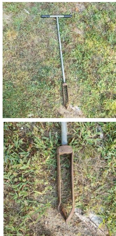
Figure 3: Photos of the auger used to collect soil samples.
