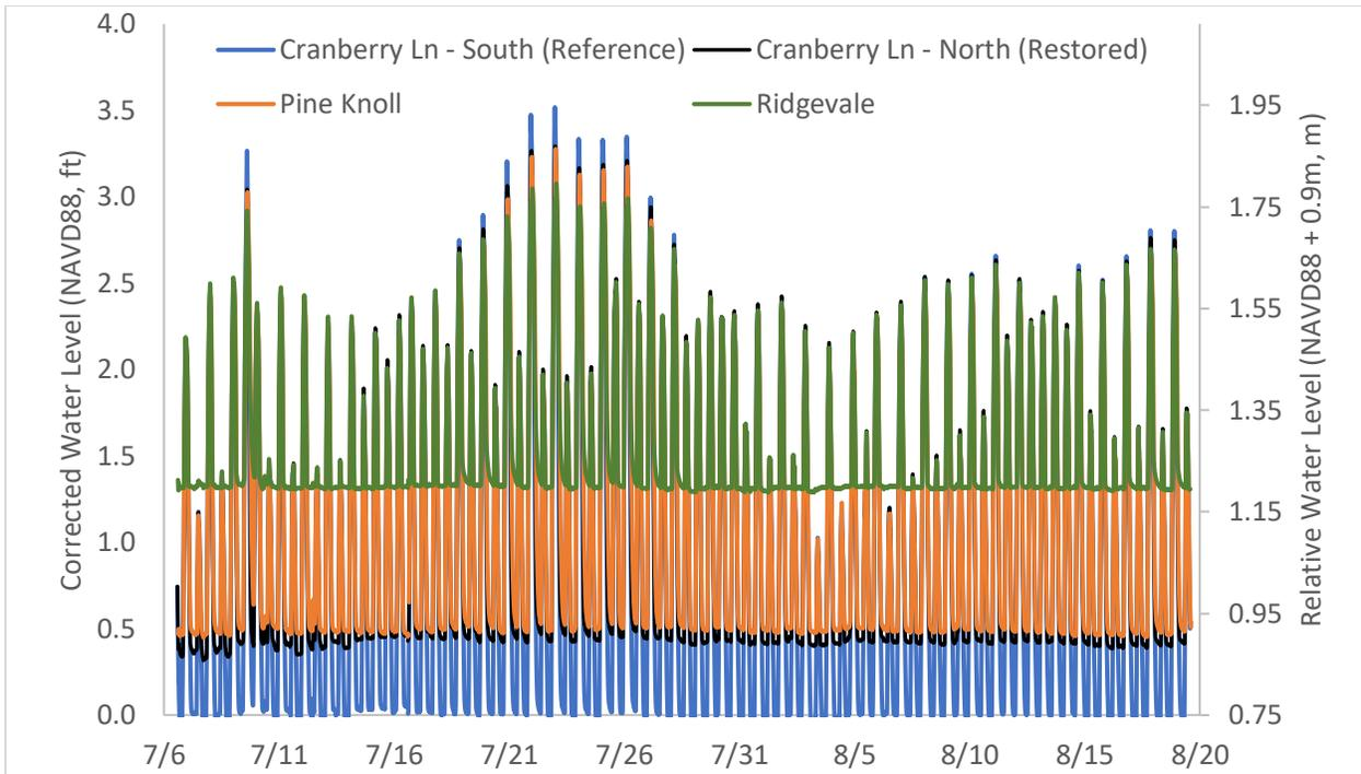
Figure 6: Water level data from four stations within the Cockle Cove and Bucks Creek marsh system. Because there was an offset during elevation data collection, the data have been corrected to NAVD88 in feet (to compare against earlier monitoring efforts). The relative water level data is also provided in meters in order to make comparisons across the other parameters collected as part of this study.
