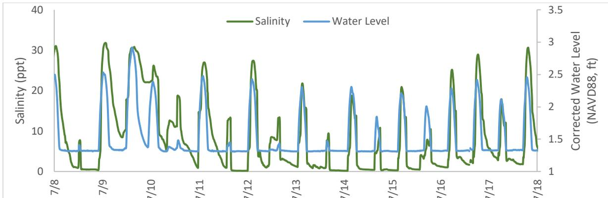
Figure 10: Salinity and water level during a neap tide at the marsh located on the western side of Ridgevale Road.
