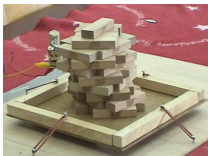
Figure 1. Sample student-designed earthquake-proof structure on earthquake simulator
